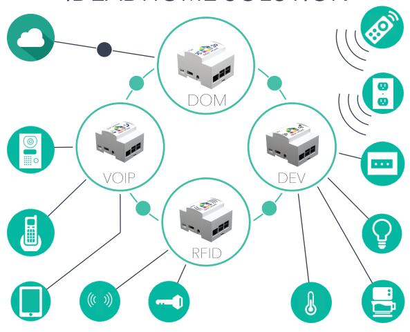
Control unit for Idea Dhome automation solution. Manages the local and remote web interface of the system and controls all the peripheral boards and cards.
