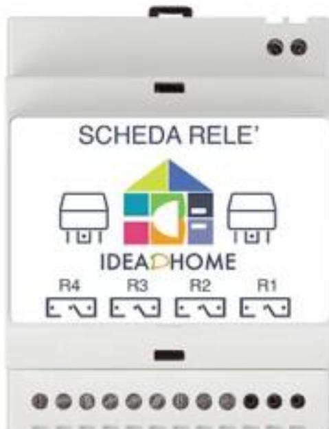
**Power Supply:** 5V DC / 400mA (relay all ON)
